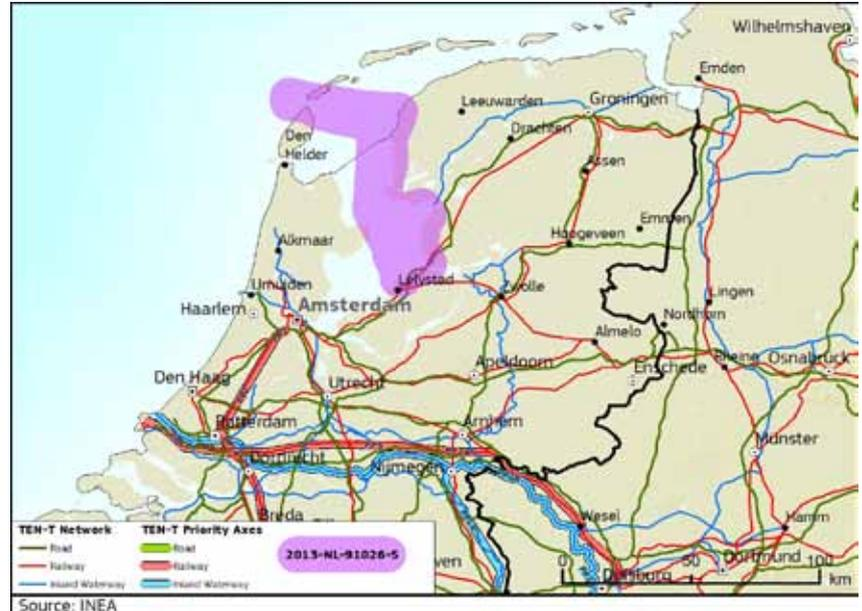
The proposed Action addresses bottlenecks on the corridor North Sea-IJsselmeer that prevent the optimal use of the waterway. The Lorentz Locks, in the Afsluitdijk, are outdated and their size doesn't allow the traffic of large container vessels and coasters. Similarly, the depth of the IJsselmeer waterway is not sufficient for container vessels and coasters.
