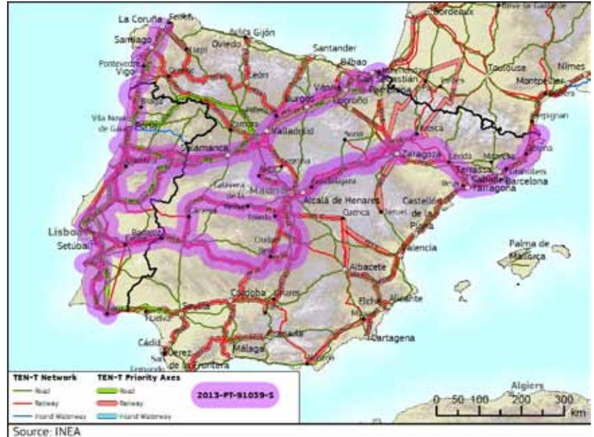
The proposed Action is part of a Global Project involving the development of a high-capacity freight and passenger railway axis linking Portugal to Spain and via France to the rest of Europe. It is a study to define the technical norms which, when implemented, will allow a three rail track system to be developed to enable both standard and Iberian gauge trains to operate on the same route, thus ensuring the gradual implementation of interoperable railway lines.
