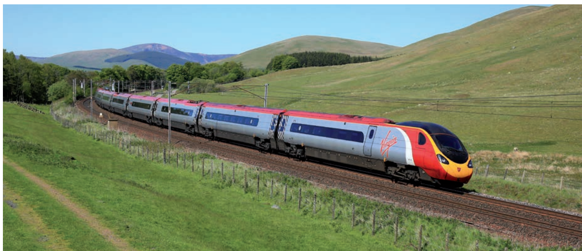
An Alstom Virgin Trains West Coast Type F Class 390 'Pendolino' train introduced in 2001
