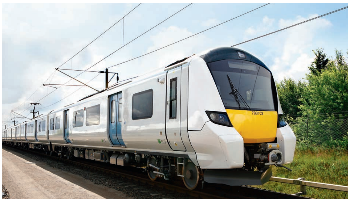
A Siemens Type E Class 700 ‘Desiro City’ EMU, to be introduced on the GoVia Thameslink routes from 2016
