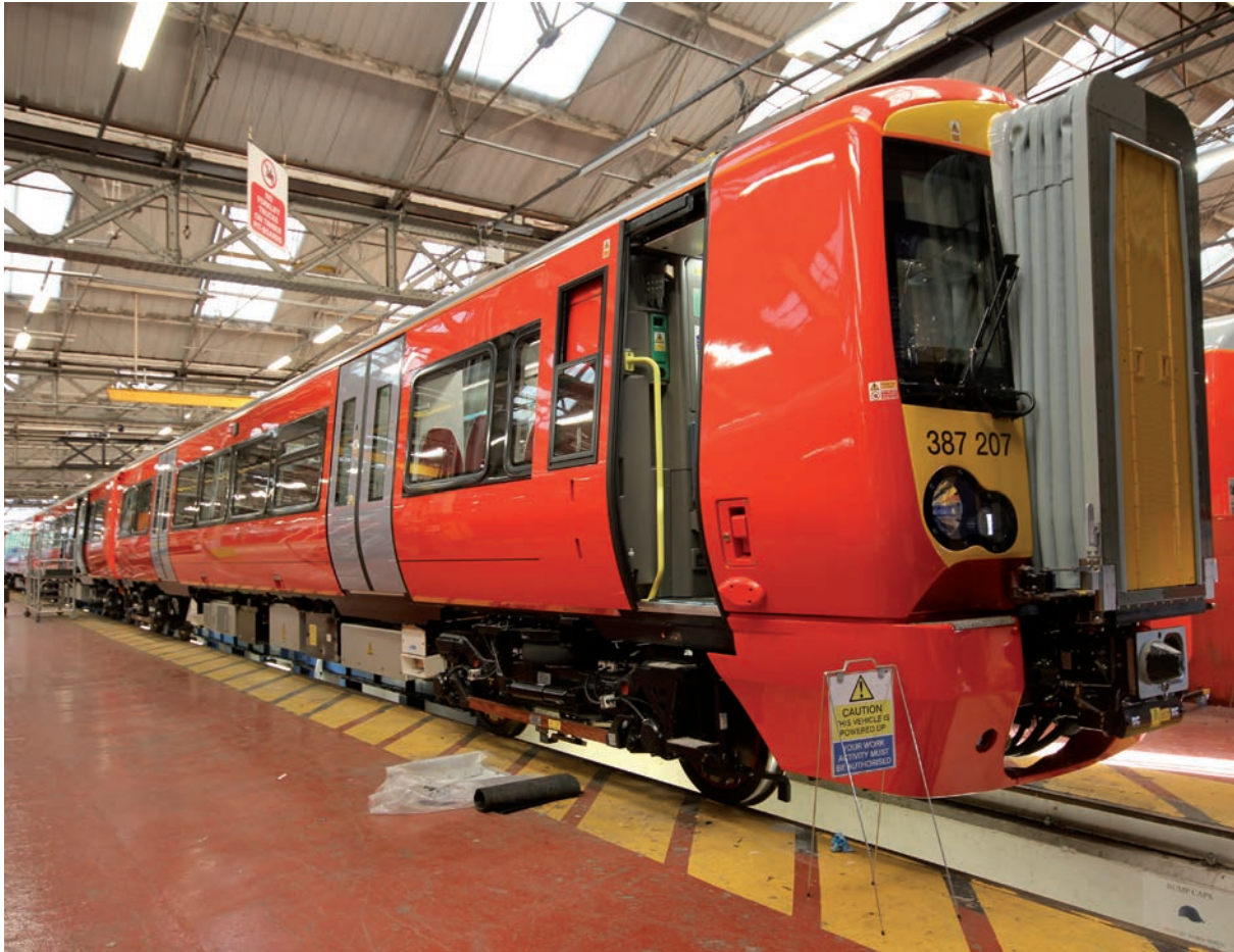
A Bombardier Type E Class 387/2 'Electrostar' EMU under construction at Derby Litchurch Lane Works for introduction on GoVia's Gatwick Express services in 2016
