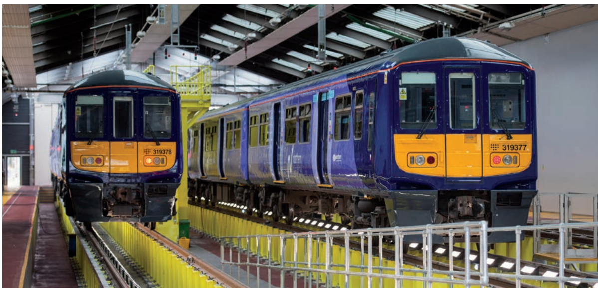
BR-procured Northern Rail Type E Class 319 EMUs introduced in 1987, at Liverpool Allerton depot
