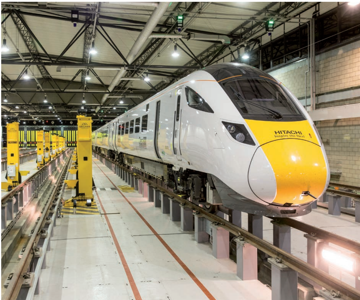
A Hitachi Type F Class 800 bi-mode 'Super Express Train', to be introduced on the Great Western Railway from 2017, at North Pole depot in West London
