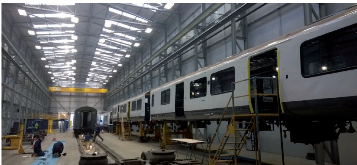
A BR-procured Abellio Greater Anglia Type E Class 321 EMU introduced in 1988, being life-extended to the 'Renatus' specification by Wabtec at Doncaster
